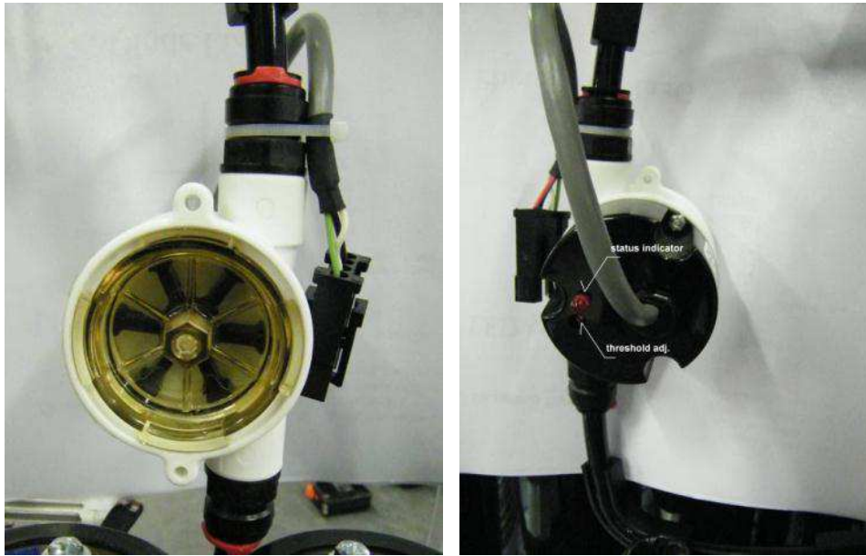
Flow switch: front and rear view.
