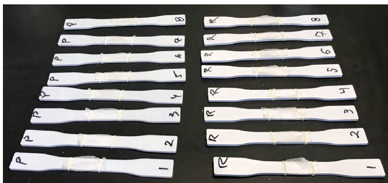
Figure 2. Raw sample stock of two materials prior to testing: (Left) Polycarbonate (Right) Custom-blended plastic used in Verathon BladderScan i10
