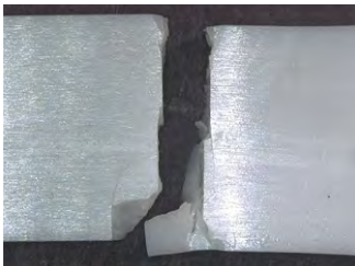
Figure 5. Top view of broken polycarbonate (Sample 4); 10x magnification.
